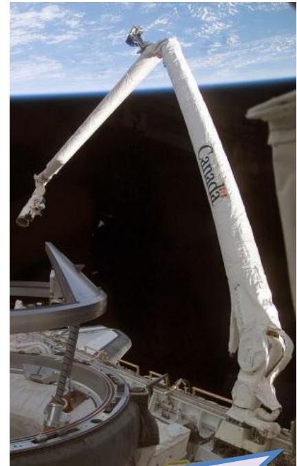
Figure -5-This robot arm takes a place on the international space station and it is used for maintenance and moving parts.
