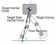
Target ZMP=Center of Ground Reaction
