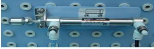
(a) Double acting cylinder
