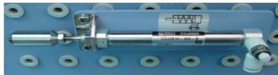
(a) Single acting cylinder
